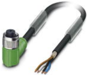
Sensor/actuator cable, 4-position, PUR halogen-free, black-gray RAL 7021, shielded, free cable end, on Socket angled M12, A-coded, cable length: 20 m
