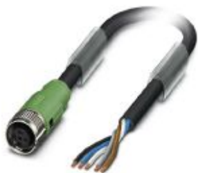
Sensor/actuator cable, 5-position, PUR, black-gray RAL 7021, free cable end, on Socket straight M12 SPEEDCON, coding: A, cable length: 15 m
