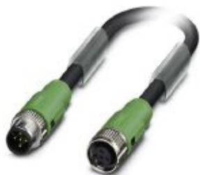
Sensor/actuator cable, 5-position, PUR, black-gray RAL 7021, Plug straight M12 SPEEDCON, coding: A, on Socket straight M12 SPEEDCON, coding: A, cable length: 1 m
