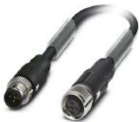
Sensor/actuator cable, 5-position, PUR halogen-free, black-gray RAL 7021, shielded, Plug straight M12 SPEEDCON, coding: B, on Socket straight M12 SPEEDCON, coding: B, cable length: 0.13 m
