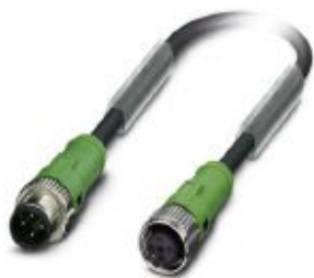
Sensor/actuator cable, 4-position, PUR halogen-free, black-gray RAL 7021, Plug straight M12 SPEEDCON, coding: A, on Socket straight M12 SPEEDCON, coding: A, cable length: 1.5 m
