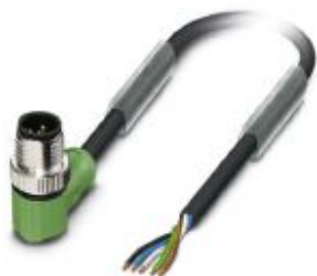
Sensor/actuator cable, 5-position, PUR halogen-free, black-gray RAL 7021, Plug angled M12 SPEEDCON, coding: A, on free cable end, cable length: 5 m
