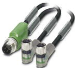
Sensor/actuator cable, 3-position, PUR, black-gray RAL 7021, Plug straight M12, A-coded, on Socket angled M8, with 2 LEDs and Socket angled M8, A-coded, with 2 LEDs, cable length: 2 m
