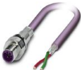
Bus system flush-type plug, PROFIBUS, 2-pos., M12, shielded, B-coded, front/screw mounting with M16 thread, with 2 m bus cable, 2 x 0.25 mm 2
