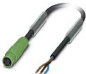
Sensor/actuator cable, 3-position, PUR halogen-free, black-gray RAL 7021, free cable end, on Socket straight M8 Snap-in, cable length: 5 m
