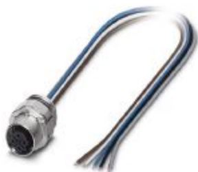
Fieldbus flush-type socket, INTERBUS/PROFIBUS, 5-pos., M12 SPEEDCON, B-coded, front/screw mounting with M16 thread, can be positioned, with 0.5 m TPE litz wire, 5x0.25 mm 2
