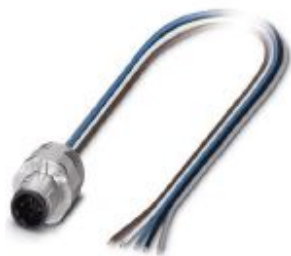
Fieldbus flush-type plug, INTERBUS/PROFIBUS, 5-pos., M12 SPEEDCON, B-coded, front/screw mounting with M16 thread, can be positioned, with 0.5 m TPE litz wire, 5x0.25 mm 2
