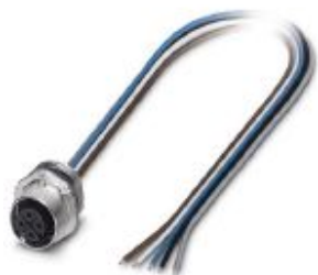
Sensor/Actuator flush-type socket, 5-pos., M12-SPEEDCON, A-coded, front/screw mounting with M16 thread, with 0.5 m TPE litz wire, 5 x 0.25 mm 2
