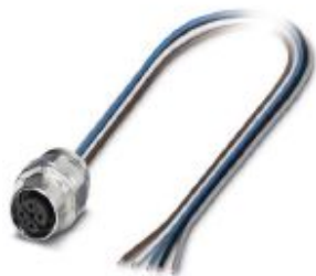
Sensor/Actuator flush-type socket, 5-pos., M12-SPEEDCON, A-coded, front/screw mounting with M16 thread, can be positioned, with 0.5 m TPE litz wire, 5 x 0.34 mm 2
