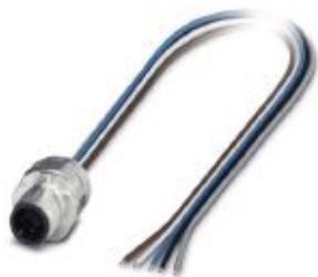
Sensor/Actuator flush-type plug, 5-pos., M12-SPEEDCON, A-coded, front/screw mounting with M16 thread, can be positioned, with 0.5 m TPE litz wire, 5 x 0.34 mm 2
