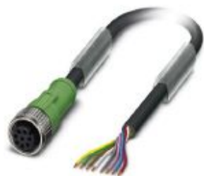
Sensor/actuator cable, 8-position, PUR halogen-free, black-gray RAL 7021, free cable end, on Socket straight M12, coding: A, cable length: 10 m
