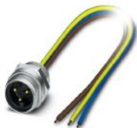
Sensor/actuator flush-type plug, 3-pos., 7/8", front mounting with Pg13.5 thread, with 0.5 m PVC litz wire, 3 x 0.75 mm 2
