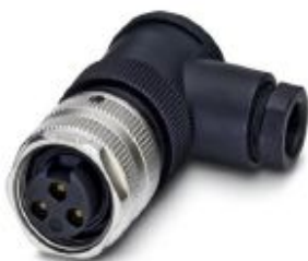
Connector, Universal, 3-position, Socket angled 7/8"-UNF, Coding: A, Screw connection, knurl material: Zinc die-cast, nickel-plated, cable gland Pg9, external cable diameter 6 mm ... 8 mm
