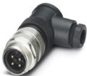
Connector, Universal, 4-position, Plug angled 7/8"-UNF, Coding: A, Screw connection, knurl material: Zinc die-cast, nickel-plated, cable gland Pg9, external cable diameter 6 mm ... 8 mm, Contact 4 leading
