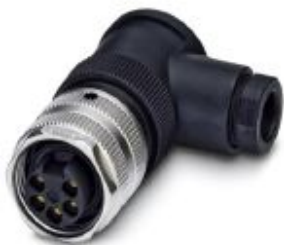
Connector, Universal, 5-position, Socket angled 7/8"-UNF, Coding: A, Screw connection, knurl material: Zinc die-cast, nickel-plated, cable gland Pg9, external cable diameter 6 mm ... 8 mm
