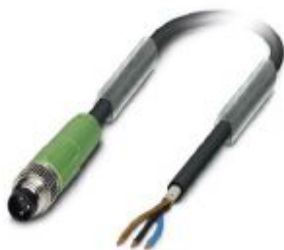
Sensor/actuator cable, 3-position, PUR halogen-free, black-gray RAL 7021, shielded, Plug straight M8, on free cable end, cable length: 10 m
