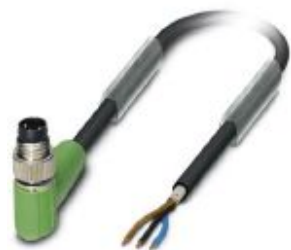
Sensor/actuator cable, 3-position, PUR halogen-free, black-gray RAL 7021, shielded, Plug angled M8, on free cable end, cable length: 5 m
