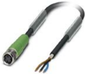
Sensor/actuator cable, 3-position, PUR halogen-free, black-gray RAL 7021, shielded, free cable end, on Socket straight M8, cable length: 1.5 m
