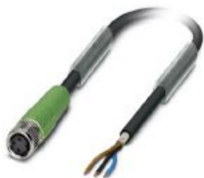
Sensor/actuator cable, 3-position, PUR halogen-free, black-gray RAL 7021, shielded, free cable end, on Socket straight M8, cable length: 10 m
