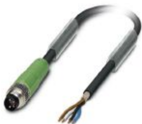
Sensor/actuator cable, 4-position, PUR halogen-free, black-gray RAL 7021, shielded, Plug straight M8, on free cable end, cable length: 1.5 m
