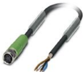
Sensor/actuator cable, 4-position, PUR halogen-free, black-gray RAL 7021, shielded, free cable end, on Socket straight M8, cable length: 10 m
