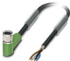
Sensor/actuator cable, 4-position, PUR halogen-free, black-gray RAL 7021, shielded, free cable end, on Socket angled M8, cable length: 1.5 m
