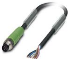
Sensor/actuator cable, 6-position, PUR halogen-free, black-gray RAL 7021, Plug straight M8, on free cable end, cable length: 3 m
