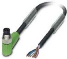
Sensor/actuator cable, 6-position, PUR halogen-free, black-gray RAL 7021, Plug angled M8, on free cable end, cable length: 5 m
