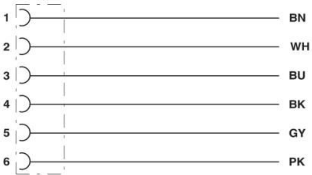
Contact assignment of M8 socket
