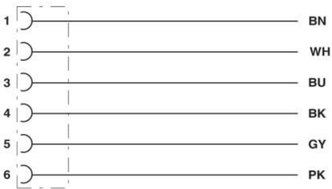
Contact assignment of M8 socket
