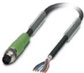
Sensor/actuator cable, 6-position, PUR halogen-free, black-gray RAL 7021, shielded, Plug straight M8, on free cable end, cable length: 3 m
