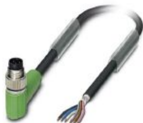
Sensor/actuator cable, 6-position, PUR halogen-free, black-gray RAL 7021, shielded, Plug angled M8, on free cable end, cable length: 3 m
