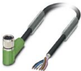
Sensor/actuator cable, 6-position, PUR halogen-free, black-gray RAL 7021, shielded, free cable end, on Socket angled M8, cable length: 1.5 m
