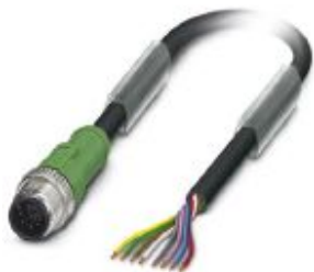
Sensor/actuator cable, 8-position, PUR halogen-free, black-gray RAL 7021, Plug straight M12, coding: A, on free cable end, cable length: 3 m
