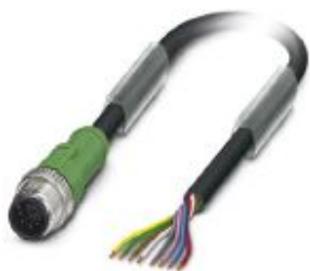
Sensor/actuator cable, 8-position, PUR halogen-free, black-gray RAL 7021, Plug straight M12, coding: A, on free cable end, cable length: 10 m
