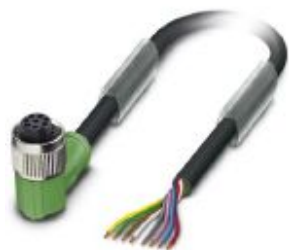
Sensor/actuator cable, 8-position, PUR halogen-free, black-gray RAL 7021, free cable end, on Socket angled M12, coding: A, cable length: 3 m
