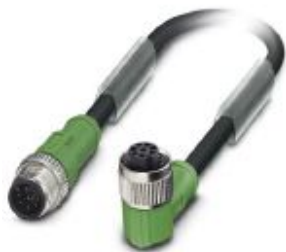
Sensor/actuator cable, 8-position, PUR halogen-free, black-gray RAL 7021, Plug straight M12, coding: A, on Socket angled M12, coding: A, cable length: 3 m
