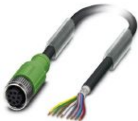
Sensor/actuator cable, 8-position, PUR halogen-free, black-gray RAL 7021, shielded, free cable end, on Socket straight M12, coding: A, cable length: 1.5 m
