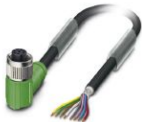
Sensor/actuator cable, 8-position, PUR halogen-free, black-gray RAL 7021, shielded, free cable end, on Socket angled M12, coding: A, cable length: 1.5 m
