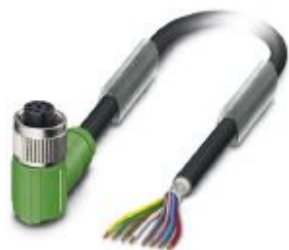
Sensor/actuator cable, 8-position, PUR halogen-free, black-gray RAL 7021, shielded, free cable end, on Socket angled M12, coding: A, cable length: 3 m
