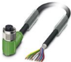
Sensor/actuator cable, 8-position, PUR halogen-free, black-gray RAL 7021, shielded, free cable end, on Socket angled M12, coding: A, cable length: 5 m
