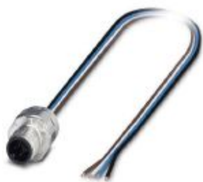
Sensor/actuator flush-type plug, 4-pos., M12 SPEEDCON, A-coded, front/screw mounting with M16 thread, can be positioned, with 0.5 m TPE litz wire, 4 x 0.34 mm 2
