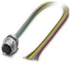
Flush-type connector, Universal, 8-position, Socket, straight, M12-SPEEDCON, A-coded, Front mounting, M16 x 1.5, Individual wires, cable length: 0.5 m, 0.25 mm 2 , TPE litz wire
