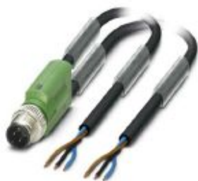
Sensor/actuator cable, 3-position, PUR halogen-free, black-gray RAL 7021, Plug straight M12 SPEEDCON, coding: A, on free cable end and free cable end, cable length: 10 m
