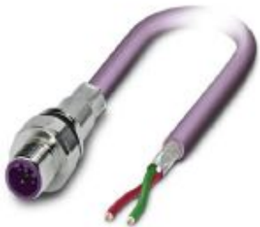
Bus system flush-type plug, PROFIBUS, 2-pos., M12, shielded, B-coded, front/screw mounting with M16 thread, with 0.5 m bus cable, 2 x 0.25 mm 2
