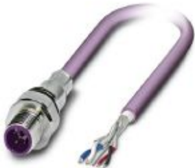
Bus system flush-type plug, DeviceNet/CANopen, 5-pos., M12, shielded, A-coded, front/screw mounting with M16 thread, with 0.5 m bus cable, 2 x 0.2 mm 2 , 2 x 0.32 mm 2
