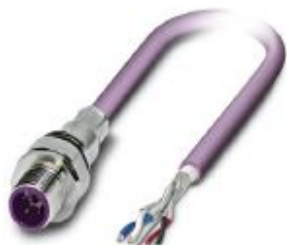
Bus system flush-type plug, DeviceNet/CANopen, 5-pos., M12, shielded, A-coded, front/screw mounting with M16 thread, with 1 m bus cable, 2 x 0.2 mm 2 , 2 x 0.32 mm 2
