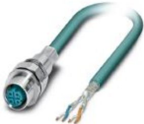
Bus system flush-type socket, Ethernet, 4-pos., M12, shielded, D-coded, front/screw mounting with M16 thread, can be positioned, with 0.5 m bus cable, 2 x 2 x 0.14 mm 2
