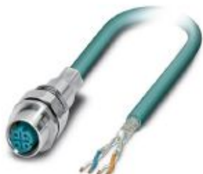
Bus system flush-type socket, Ethernet, 4-pos., M12, shielded, D-coded, front/screw mounting with M16 thread, can be positioned, with 5 m bus cable, 2 x 2 x 0.14 mm 2
