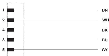
Contact assignment of the M12 socket
